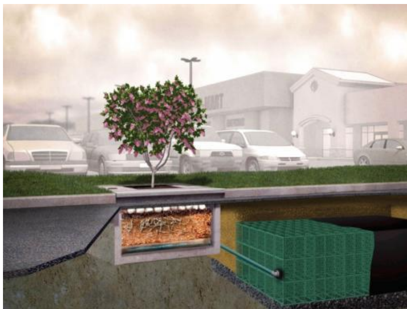
Figure 3 Example of tree pit drainage system - from 'Sustainable Drainage - Retrofitting the Built Environment' by Arup
