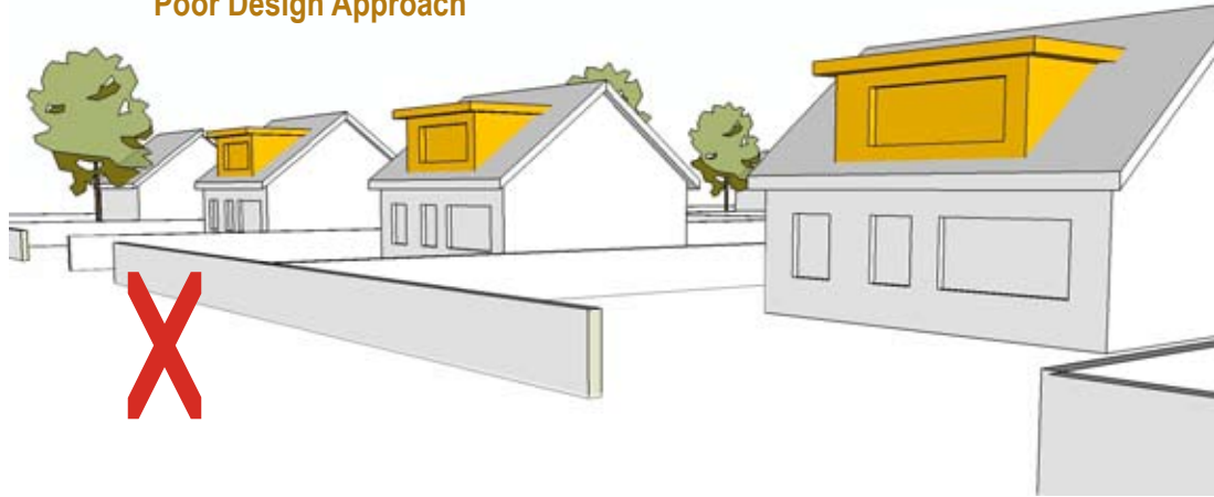
Design Guidance 6: Potential Impact of Front Dormer on Streetscape - Poor Design Approach
