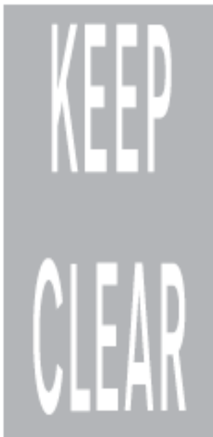
Do not block that part of the carriageway indicated
