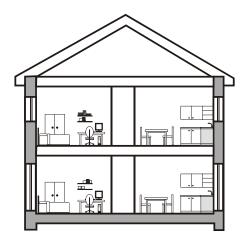
**Buffer Zones**: Non-habitable rooms within student cluster flats such as halls can be used as buffer zones to 'absorb' noise. Storage space in adjoining rooms can also be used to provide this buffering function.
