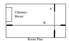
In a room, measure the distances of A & B and multiply together to work out the floor area. (The space taken by the chimneybreast is not included as floor area).
